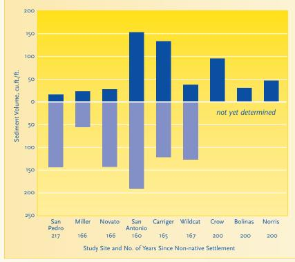
Normalized volumes of sediment supplied per linear foot of mainstem channel from either bed incision (light blue) or bank erosion (dark blue) since the time of non-native settlement, which is shown as years for each watershed ain the small boxes at the base of each graph.As can be seen, bed incision has been as important (if not more important) as bank erosion to contributing sediment to the San Francisco Estuary.
