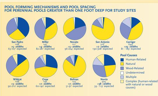
Note: Expected spacing is based upon 3 to 7 bankfull widths, which allows for a range of morphologic conditions that can include entrenched and confined channels.
