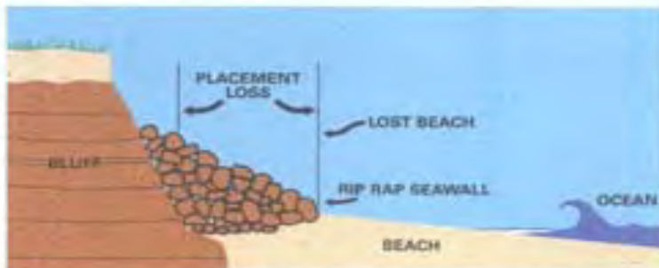
C. Placement loss of beach due to construction of a rip-rap seawall
