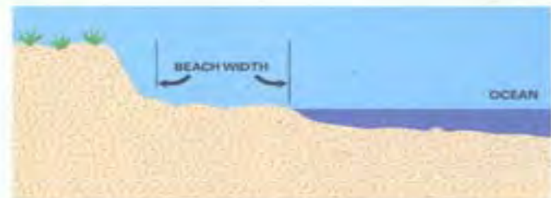
B. Shoreline after sea level rise & associated dune or bluff erosion, although the shoreline has moved landward, the beach width remains the same
