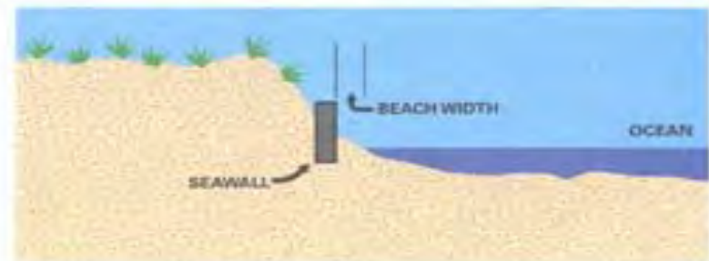
C. Shoreline after sea level rise where seawall has fixed shoreline position, note reduced beach width
